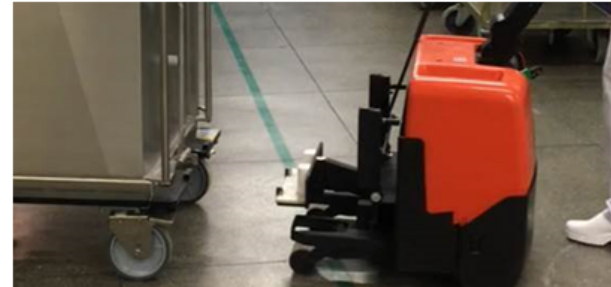
Trolley lifted at the tow bar end
